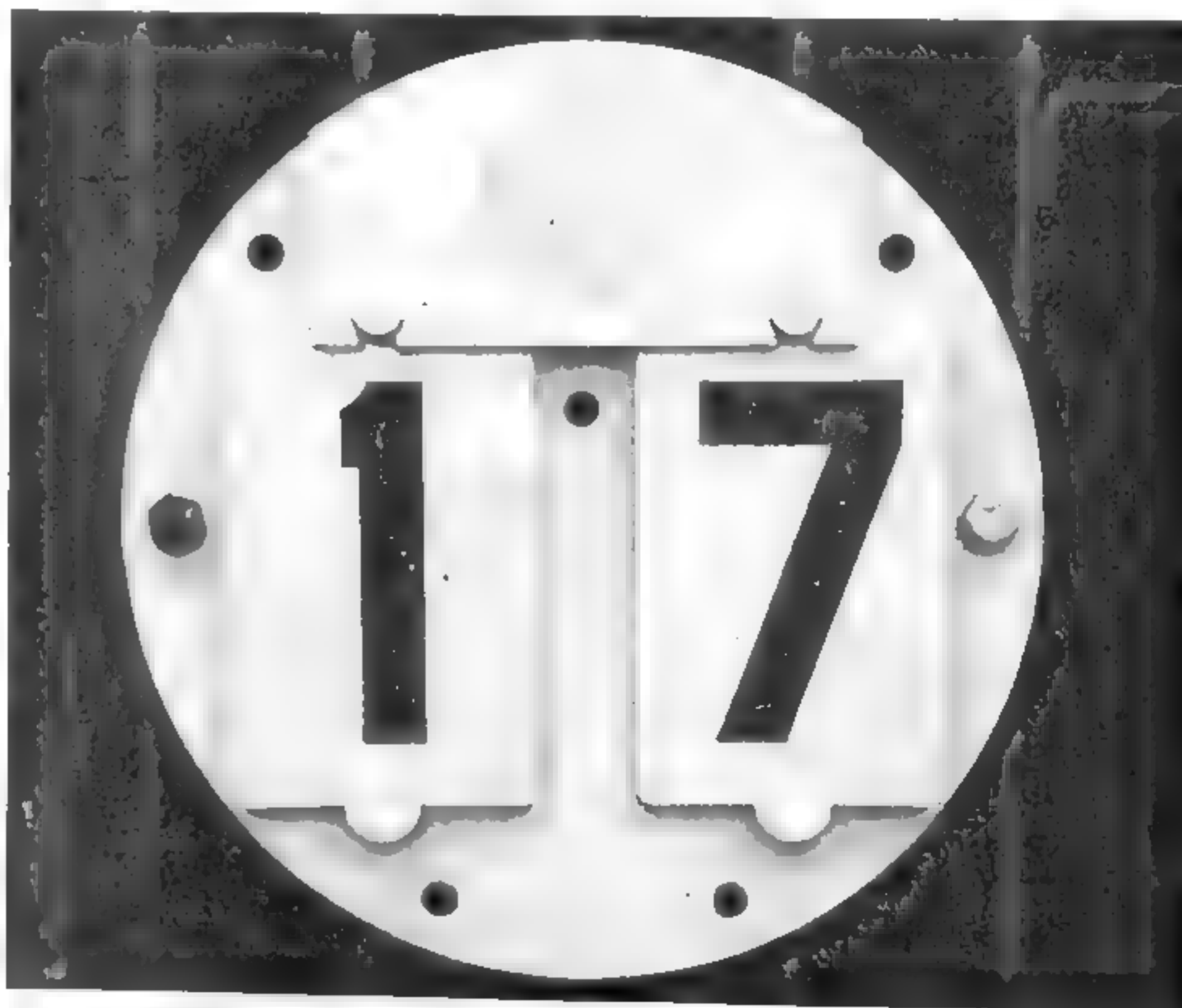
The post-WWII bridge plate featured a single line of moveable numbers, allowing it to be changed for different loads. The C was to be displayed when towing a load, indicating combination weight. When the NATO camouflage scheme came into use, the yellow bridge plates were discontinued in favor of green plates.
